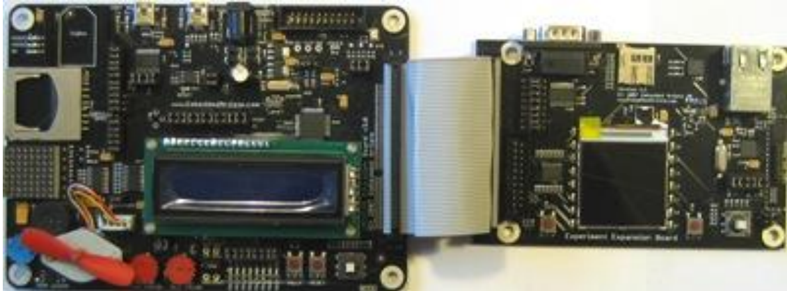
Figure 1 - LPC2148 Education Board with Experiment Expansion Board
